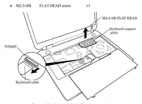
Figure 4-12 Removing the keyboard support plate
